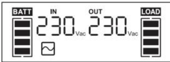
Fig. 9. Display in normal mode.
