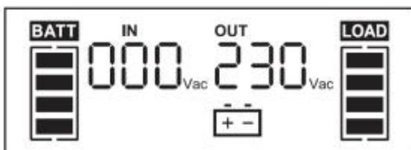
Fig. 11. Display in battery mode.
